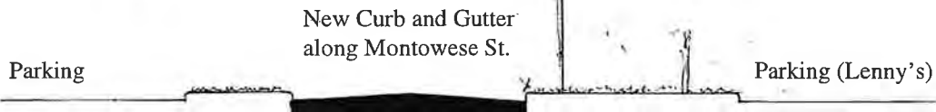
Figure 69 - Concept plan illustrates the use of shared driveways and curb control to reduce turning movements to and from Montowese Street.
